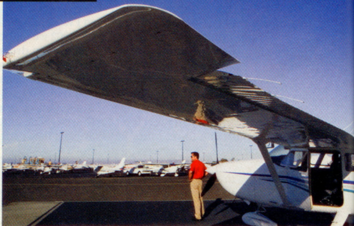
The LoPresti HID Boom Beam lights have been a safety boon (above). The wing extensions improve slow-flight characteristics (right).
