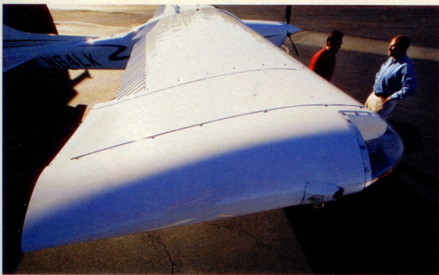
Modifications to the Skylane include a 3-foot wing extension by Wing-X STOL and wing tips by RMB.
